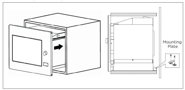
• Open the door, fix the oven to the cabinet with Screw, at the installation hole.
